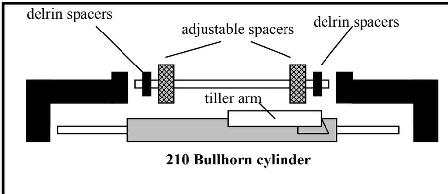
1) Lay out all the parts on a clean sheet of paper or bench and assemble the two horns onto the piston rod. Simply place the horn casting onto the piston rod as shown above, fit the washers and the Nylock nuts. Tighten them firmly, using a spanner on each end of the piston rod and ensuring that the horns stay flat on the bench. This keeps them in the same plane. **Carefully read and follow** any instructions, or warnings, included with the cylinder.
