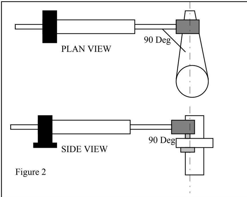
A typical single rudder installation is shown in Fig.2 above. The rudder should be in-line with the tiller arm, and the slave cylinder should be mounted squarely to the tiller arm. Please also note that the cylinder should be both square and parallel to the tiller arm.
